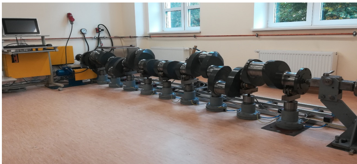
Figure 2. The test rig operating in line with the concept of the measuring system with flexible support of a crankshaft (own source).
