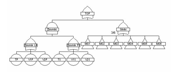
Fig.6. A fault tree for the fuel system of the generating set engines – valves separating power plants are open
