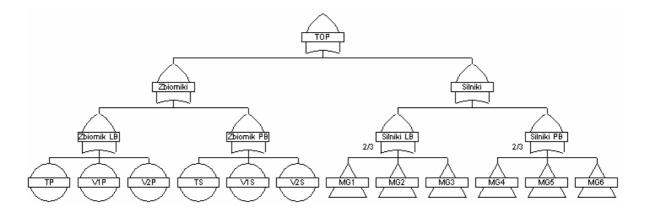
Fig. 7. A fault tree for the fuel system of the main generating set engines – valves separating power plants are closed
