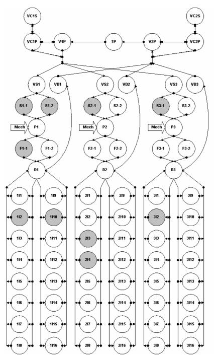
Fig. 4. Functional structure of energetic fluids flow in the port main engine room fuel supply system
