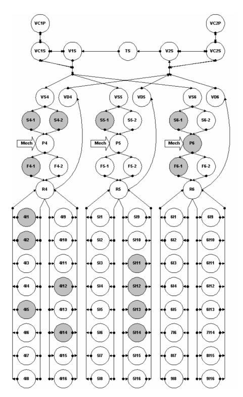
Fig. 5. Functional structure of energetic fluids flow in the starboard main engine room fuel supply system
