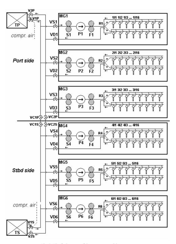
Fig. 3. The fuel system of the power-propulsion system
